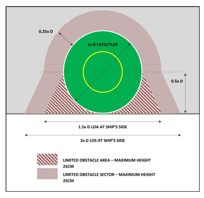
Figure 14: Ships-side non-purpose-built shipboard heliport obstacle limitation sectors and surfaces
