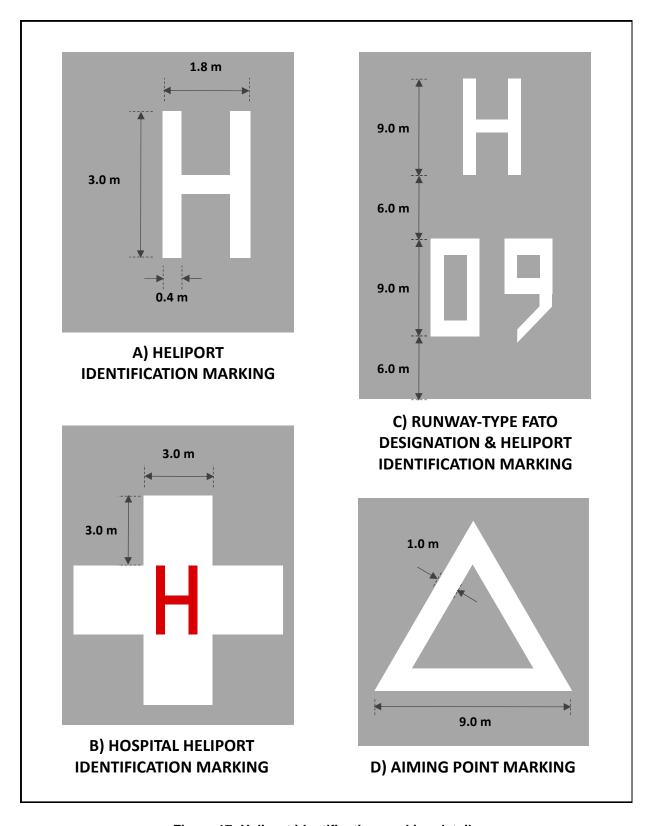
Figure 17: Heliport identification marking details
