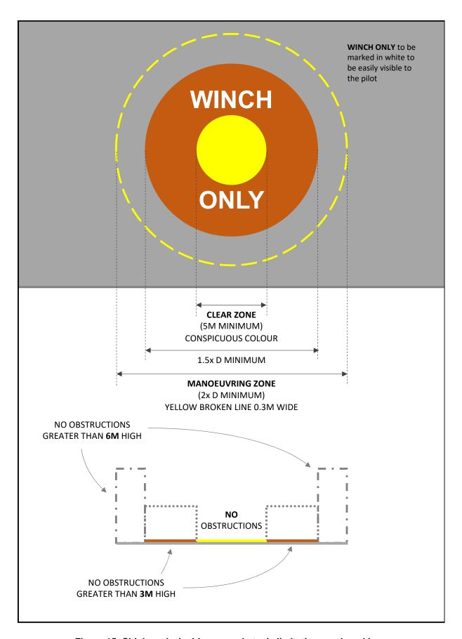
Figure 15: Shipboard winching area obstacle limitations and markings
