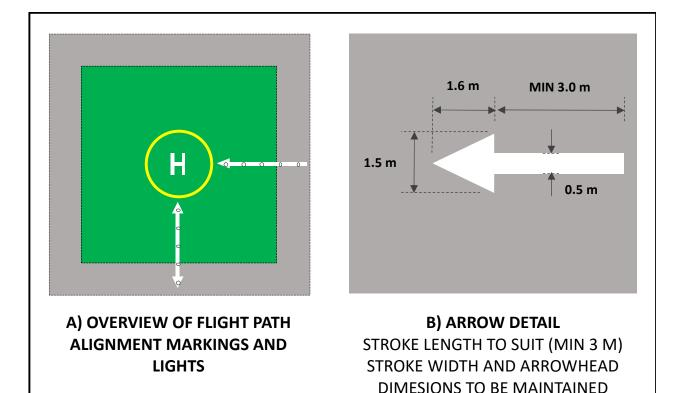
Figure 21: Flight path alignment guidance markings and lights
