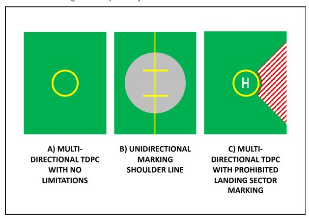
Figure 19: Examples of touchdown/positioning markings
