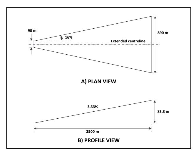
Figure 8: Approach surface for non-precision approach FATOs
