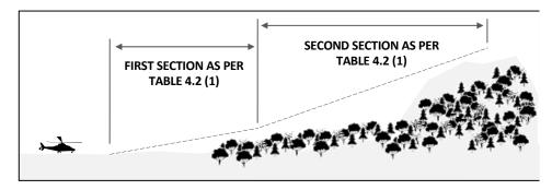
B) APPROACH AND TAKE-OFF CLIMB SURFACES - "B" SLOPE PROFILE - 8% & 16% DESIGN
