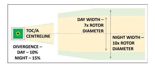
Figure 6: Overview of take-off climb/approach surface for non-instrument FATOs
