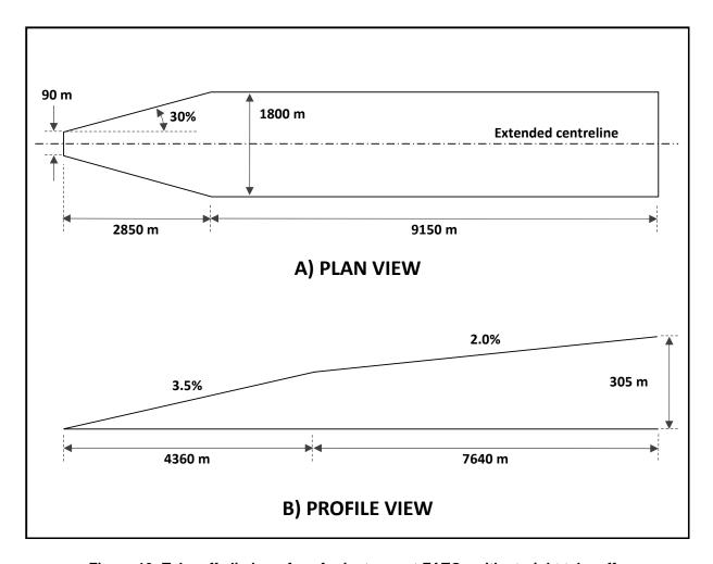
Figure 10: Take-off climb surface for instrument FATOs with straight take-offs
