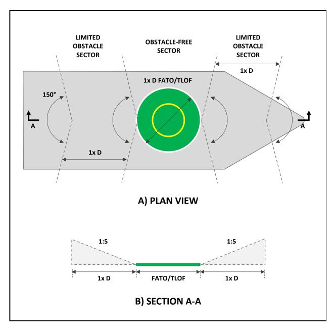
Figure 13: Amidships location - shipboard heliport obstacle limitation surfaces
